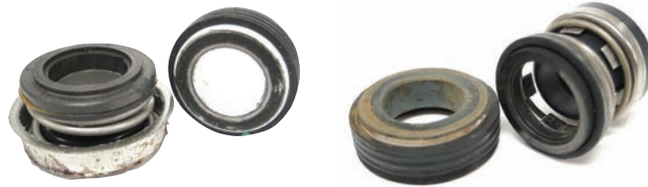
PTFE or Silicone Based Lubricants Damage Seals
